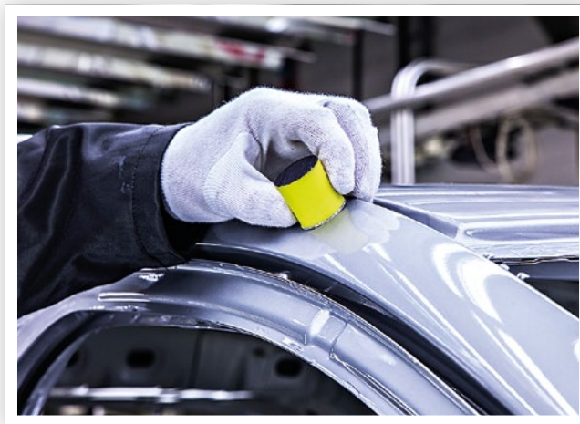
» Waterproof finessing discs enable a fast cut and a reliable finish. The product can be used wet or dry with an orbital sander or a random orbital sander.
