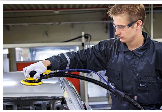
▶ Mirka® DEROS or Mirka® PROS with Abranet products or Q.Silver Ace P320–P400. Sanding on larger areas.
